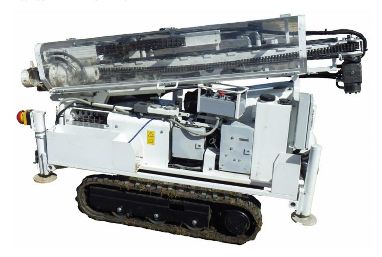
TB 175: AUGER, DESTRUCTIVE AND PRESSUREMETER BORING
