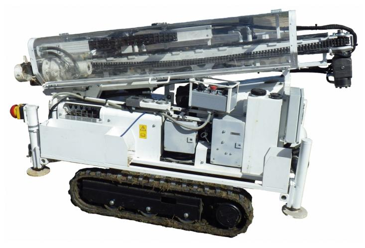
TB 175: AUGER, DESTRUCTIVE AND PRESSUREMETER BORING
